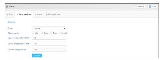
The main element configuration description of temperature alarm information interface:
