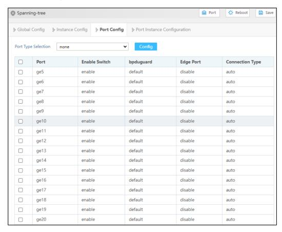
The main element configuration description of port configuration interface:
