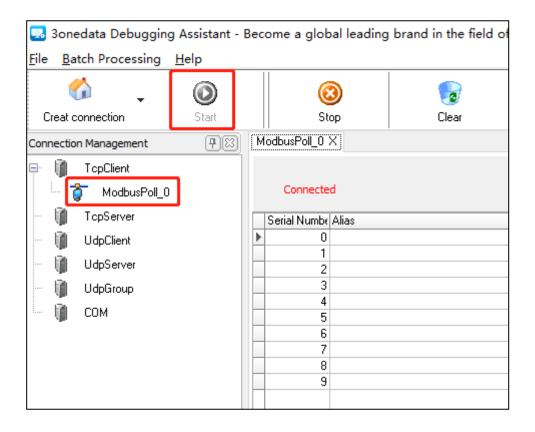
**Step 10** Check responsive data, and convert the hexadecimal value read by register into ASCII code, displayed as "Industrial Switch";
