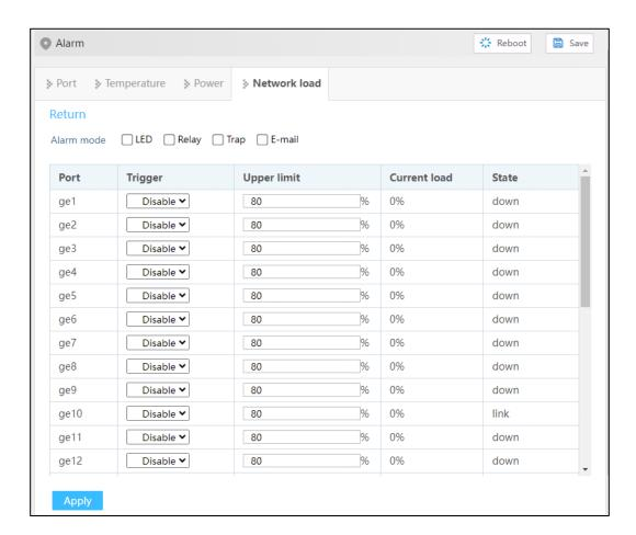
The main element configuration description of network load alarm interface:
