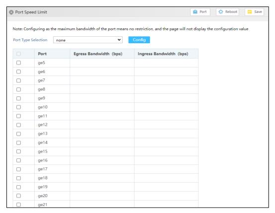
The main element configuration description of port speed limit interface:
